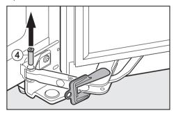
■ Push hinge pin ④ up and out from underneath.
